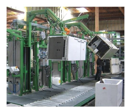
CFC refrigerant and foam blowing agents are extracted, processed and destroyed
