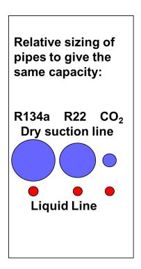
Poor thermodynamic efficiency can be offset by thermophysical gains. It means component design and system configuration have to be optimised accordingly.
