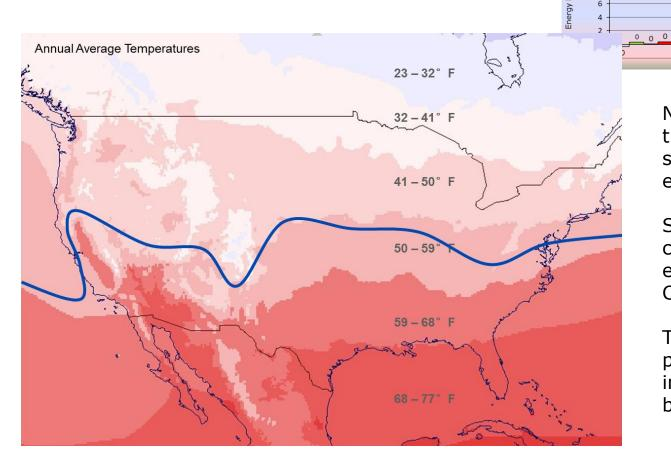
North of the blue line, transcritical CO<sub>2</sub> booster systems will have an efficiency advantage.
