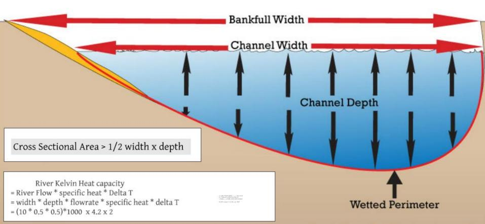
The total length of the river channel in contact with water in the cross section.
