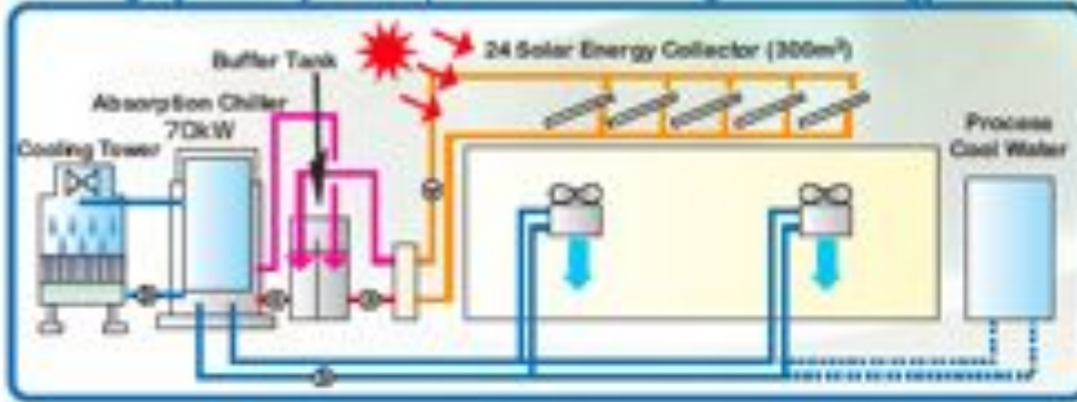
Cooling System by Adsorption Chiller Using Solar Energy
