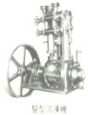
1924 Vertical low speed reciprocating refrigeration compressor
