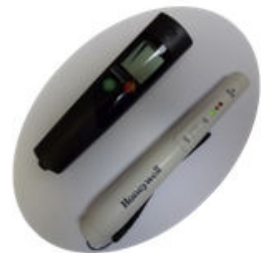
Figure 2, flammable gas detectors
