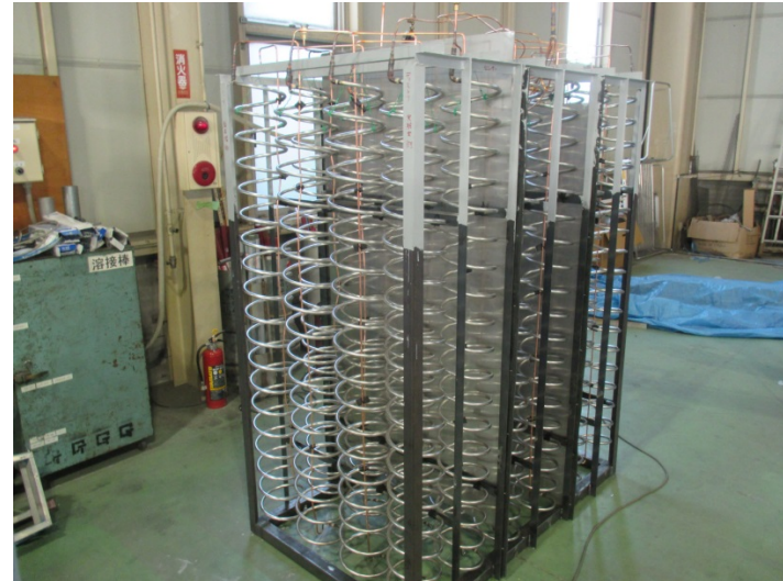
Brine-ice storage generator for CO 2
