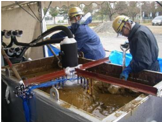
Excavation of frozen soil
