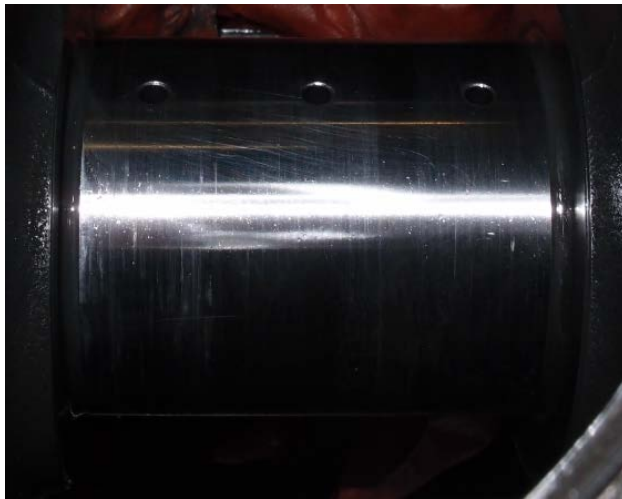
View from Piston 1 Good condition
