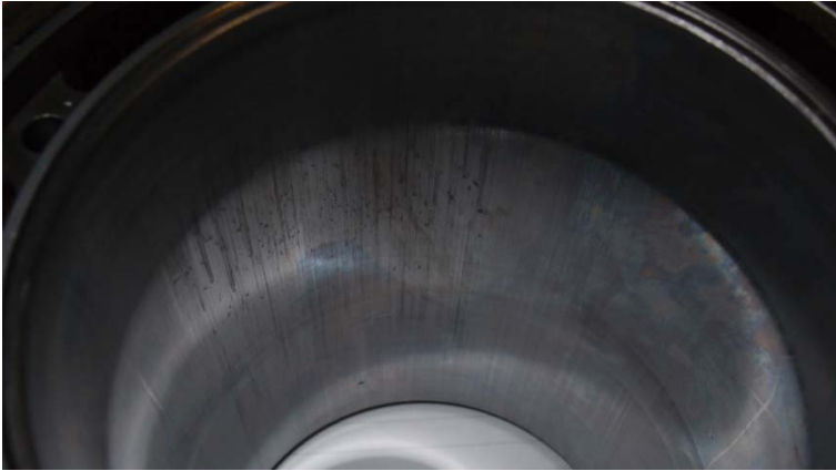
Thrust side Good condition Limited scratched area
