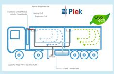
Cryogenic indirect and open loop using R744
