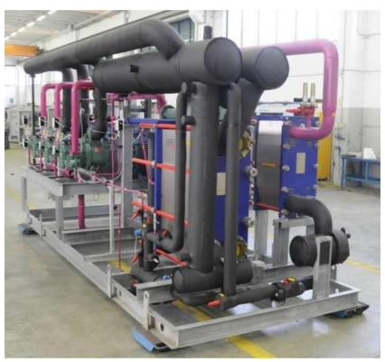
SCM new range of NH<sub>3</sub> units for indoor installation with the following features:
