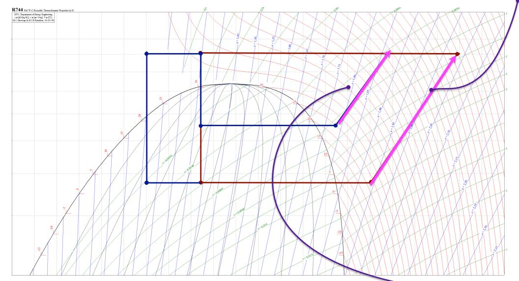
**✓ 1 PISTON WORKS BETWEEN INTERMEDIATE PRESSURE AND HIGH PRESSURE**
