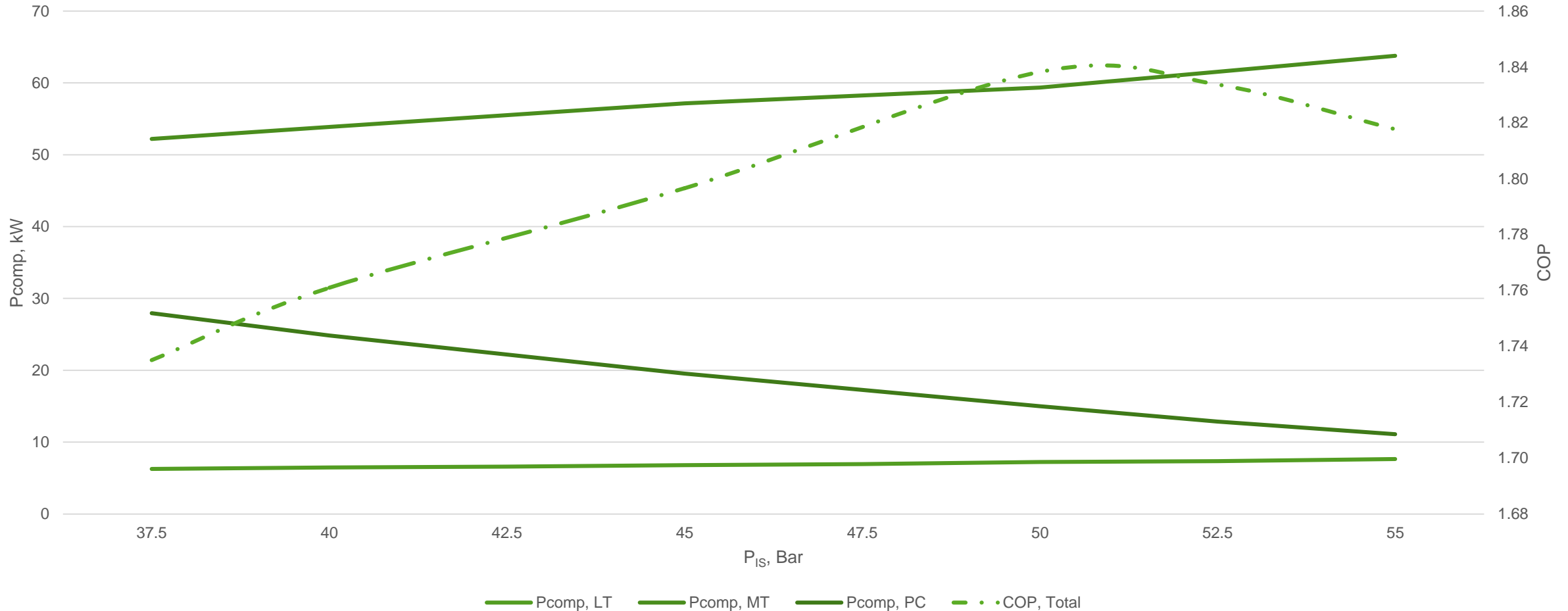
Affect of Deviation of Interstage Pressure 35C GCLT, 75% MT, 25% LT
