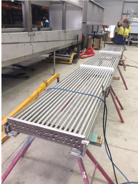
Figure 7 - Assembly of Condensing Tube Bundle. Twelve/Condenser.
