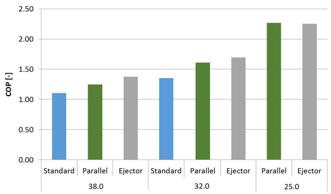
An average 7% increased efficiency in addition to the parallel compressor operation is expected
