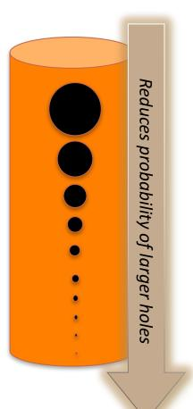
Improved tightness corresponds to lower probability of a given leak hole size
