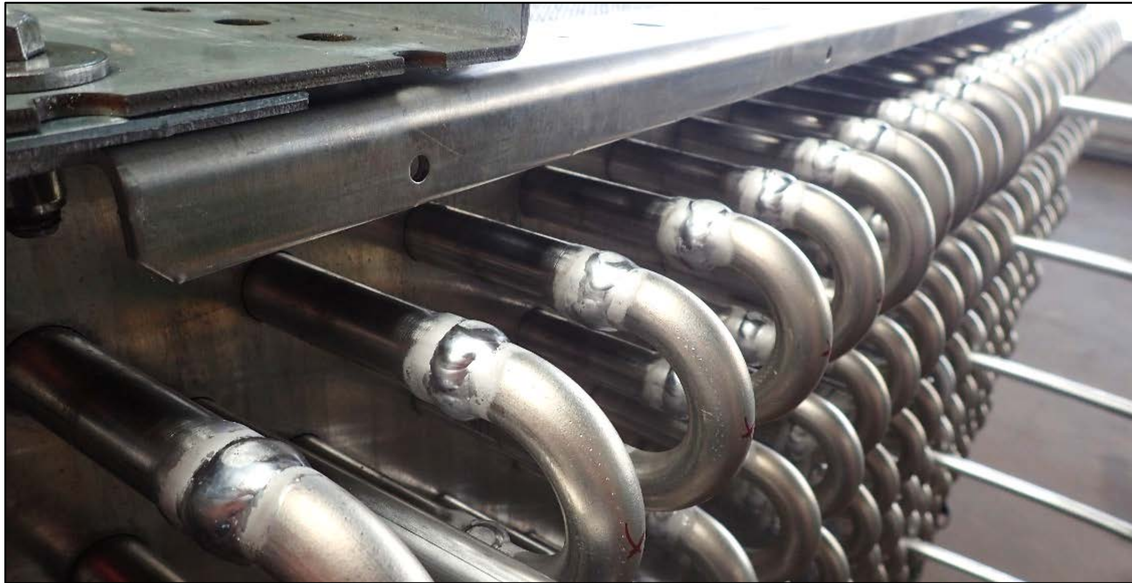
Smaller tubes for lower NH 3 inventories
