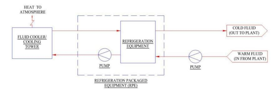
BY USING A SMALL QUANTITY OF AMMONIA TO MAKE CHILLED WATER/BRINE; SYSTEMS WITH A SECONDARY REFRIGERANT OFFER AN ALTERNATIVE TO TRADITIONAL AMMONIA SYSTEMS, OR A NATURAL ALTERNATIVE TO CENTRIFUGAL CHILLERS/FREON SYSTEMS.
