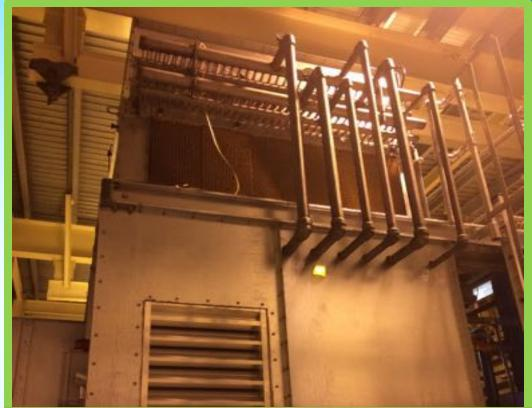
The complete unit operated at full & part loads in Evapco's Environmental Test Lab "D". Put thru extensive testing from -30°F to 100°F ambient. Unit continues to run today.
